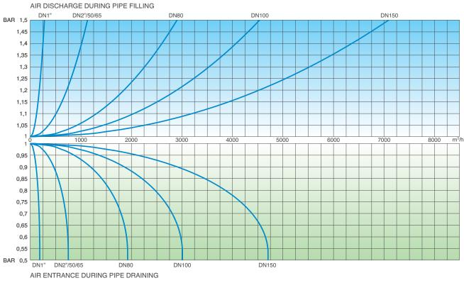
The air flow charts were created in Kg/s from laboratory tests and numerical analysis, then converted using a safety factor.
