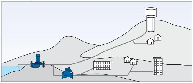
The pump supplies water to the network and to the reservoir. System pressure is too high for the residential neighborhood, requiring a pressure reducing system.
